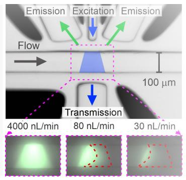
Microscope image of 490nm light impinging on a stream of fluorescein (green), which represents the area of measurement through which the activated fluorescein molecules pass. As flow rate decreases, fluorescein bleaches as it moves past the laser, resulting in less emitted light
