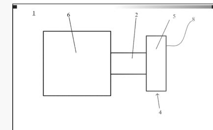
Optical meter 1 includes ref ector 4 disposed force member 2. Ref ector 4 is conf gured to receive radiation and to communicate a pressure of the radiation to force member 2. Ref ector 4 includes substrate 5 and ref ective surface 8. Force member 2 is conf gured to be displaced in response to receiving the force comprising the pressure, and optical meter 1 is conf gured to measure a power of the radiation, an energy of the radiation, or a combination thereof based on the pressure.
