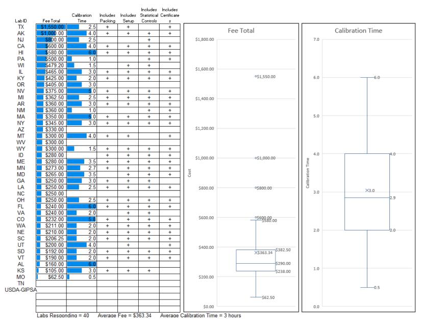
Figure 41: Fees charged for testing a set of 20 50 lb cast iron pipe-handle style test weights to NIST HB 105-1 Class F tolerances using mass echelon III procedures. 5 adjustments were assumed.
