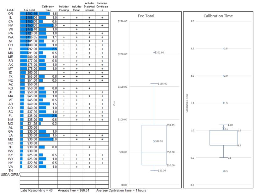
Figure 46: Fees charged for testing a 5 gallon test measure via volume transfer technique.
