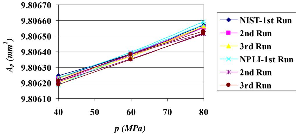
Figure 4:  $A_{p,av} (mm^2)$  of the transfer standard - NPLI-100MPN with  $p (MPa)$  against NIST PG21 and NPLI-200MPN
