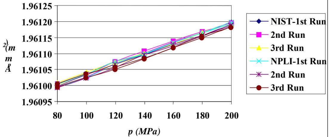
Figure 2 :  $A_{p,av} (mm^2)$  of the transfer standard - NPLI- with  $p (MPa)$  against NIST PG21 and NPLI-200MPN
