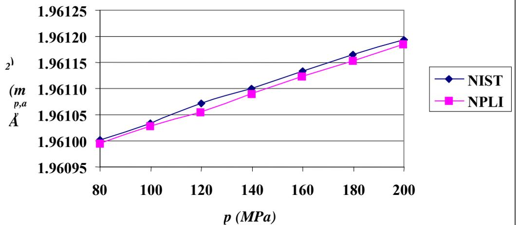
Figure 3 :  $A_p (mm^2)$  of the transfer standard - NPLI-100MPN with  $p (MPa)$  against NIST PG21 and NPLI-200MPN
