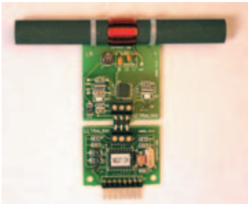
Figure 2.9. WWVB Receiver Circuit
