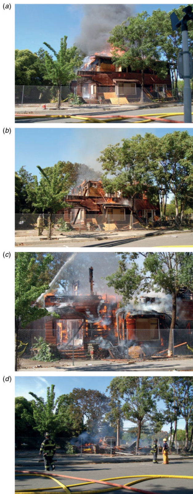
Fig. 3. Pictures of a structure during the burn: (a) 30 min after ignition; (b) 45 min after ignition; (c) 1 h 15 min after ignition and (d) 2 h after ignition.
