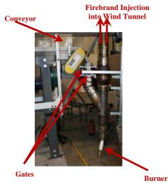
Figure 1 Schematic of NIST Continuous Feed Baby Dragon (side view) interfaced with bench scale wind tunnel.
