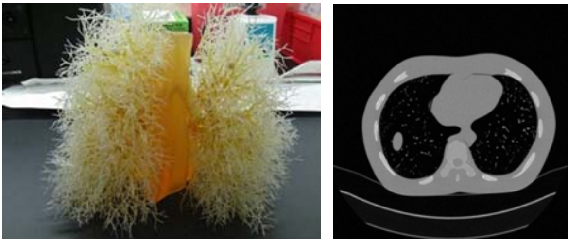
Figure 38. FDA lung phantom (left), and sample CT slice containing a phantom tumor (right).
