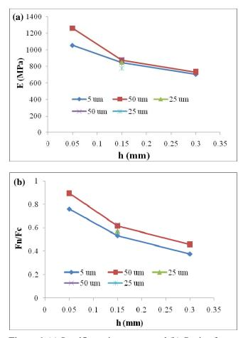
**Figure 6.** (a) Specific cutting energy, and (b) Cutting force ratio vs. uncut chip thickness, h, for different edge radii (v=5 m/s).
