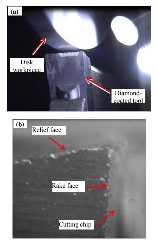
**Figure 3.** (a) Close-up view of tool and workpiece setup, and (b) Side view of a diamond-coated tool tip.
