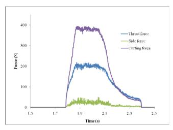
Figure 4. Cutting force history from one test.
