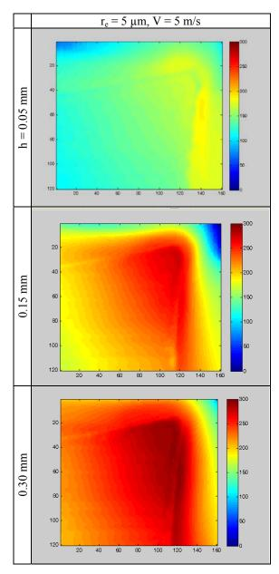
**Figure 7.** Cutting tool temperature contours (°C) at different uncut chip thicknesses, h (x and y scales in pixels).
