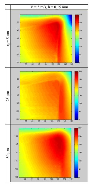
**Figure 10.** Cutting tool temperature contours (°C) at different edge radii (x and y scales in pixels).
