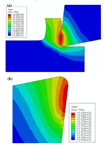
**Figure 12.** Cutting tool tip temperature contours: (a) Overall, and (b) Tool alone (Unit: °C).
