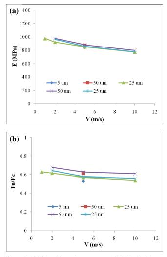
**Figure 8.** (a) Specific cutting energy, and (b) Cutting force ratio vs. cutting speed for different edge radii (h=0.15 mm).
