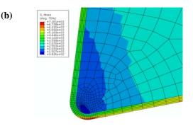
**Figure 11.** Stress contour from cutting simulations: (a) Workpiece and chip, and (b) Tool alone (unit: MPa).
