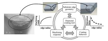
**Figure 1.** Conceptual illustration of the edge-geometry importance to diamond-coated tools for machining.
