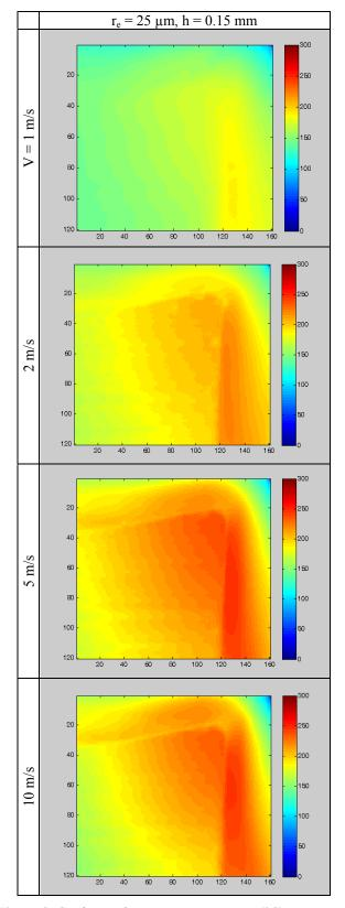
**Figure 9.** Cutting tool temperature contours (°C) at different cutting speeds (x and y scales in pixels).
