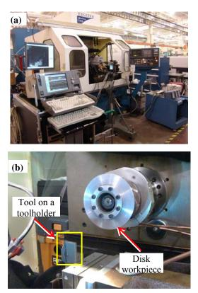
**Figure 2.** (a) 2D orthogonal cutting test-bed, and (b) Workpiece and tool arrangement in the machine.
