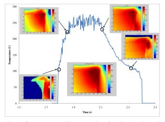
**Figure 5.** Temperature history at a location close to the tool tip; inserts are thermal images at different times.
