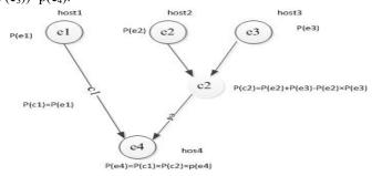
Figure2: Example Probabilistic Attack Graph
