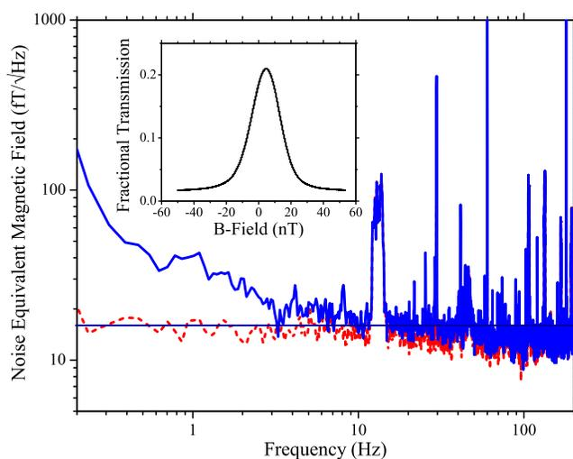
FIG. 2. Noise equivalent magnetic field measured in the sensor for the in-phase (blue solid line) and out-of-phase (red dashed line) lock-in output signals. The solid straight line shows a sensitivity of  $16 \text{ fT}/\sqrt{\text{Hz}}$ . The inset shows a typical magnetic resonance signal as the fractional optical power transmitted through the vapor cell as a function of magnetic field.
