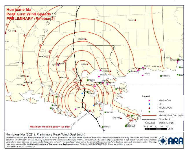
*Figure 5.* A map of preliminary peak wind gusts for Hurricane Ida in 2021 adjusted to a common exposure setting similar to an open grass field. This product was developed by NIST, in conjunction with Applied Research Associates.
