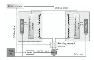
An automated comparison measurement between two PJVS systems using an analog nanovoltmeter
