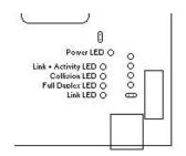
Figure 3: Network Status LEDs
