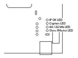
Figure 4: Microphone array Status LEDs
