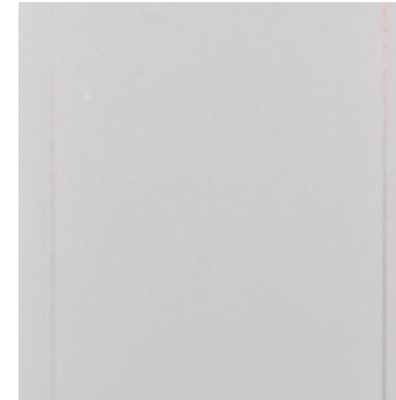
TPT™- E side - no cracking after 5000 hour air side xenon exposure
