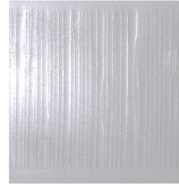
HPET1 inner tie layer cracking after 5000 hour air side xenon exposure
