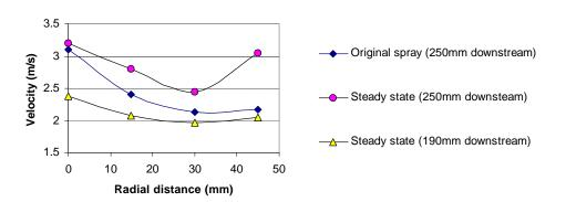
Figure 10: Velocity distributions of 0.385 g/s spray (size distribution 2), before and after the interaction at different locations.
