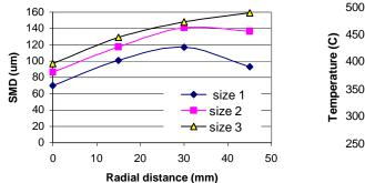
Figure 5: The initial size distributions for the three sprays at 0.385 g/s.
