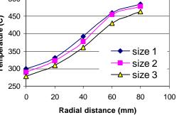
Figure 6: The steady state surface temperature profile for the three 0.385 g/s size distributions.
