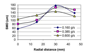
Figure 7: Size distribution of the spray in steady state, measured 250 mm downstream from the nozzle, and 4 mm above the heated plate.
