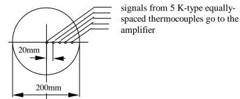
Figure 2: The structure of the heated surface with the thermocouples.
