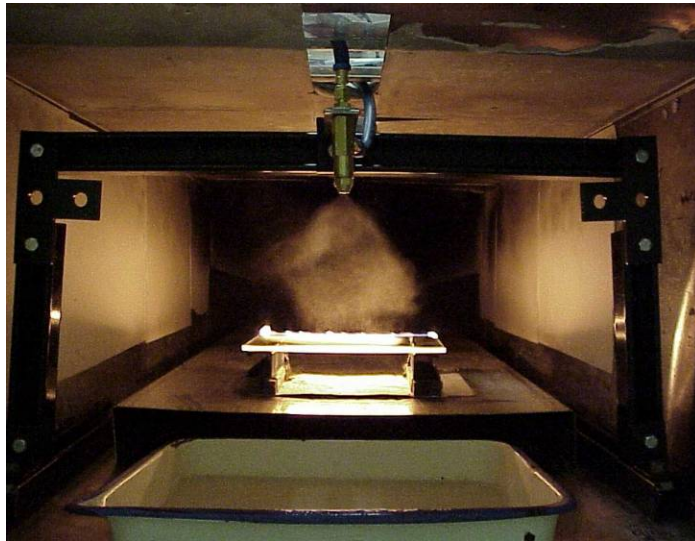
Figure 4-81. Flame Spread Experiment with Water Mist.
