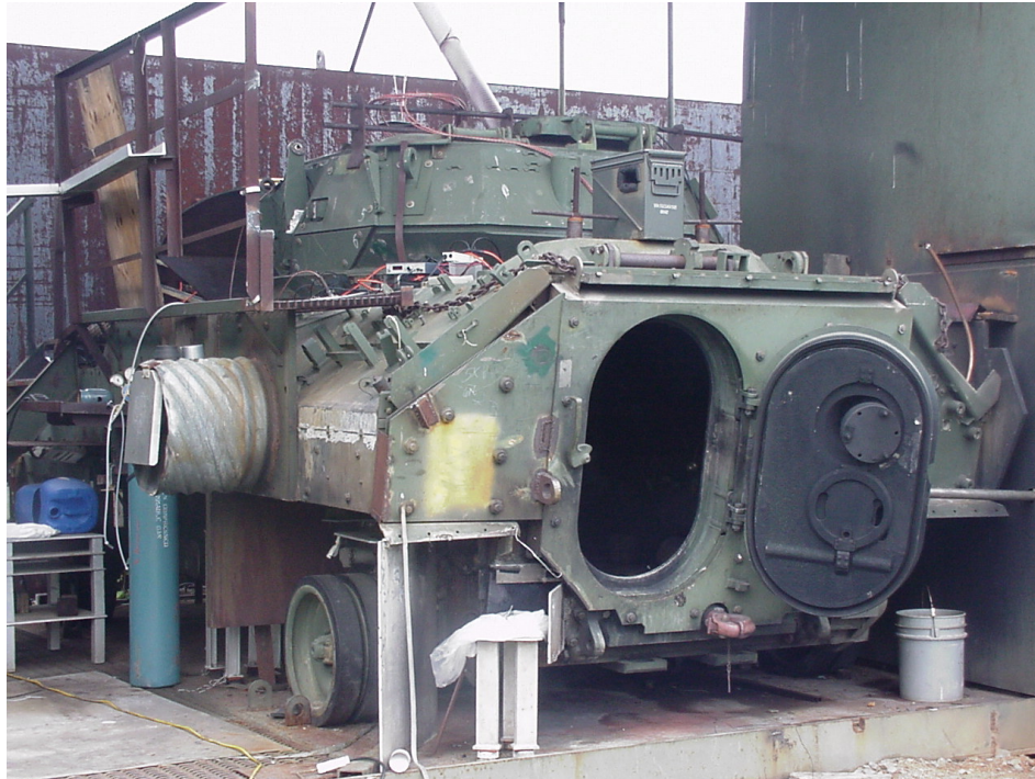
Figure 5–24. Bradley armored personnel carrier modified for performing agent release and fire suppression studies.
