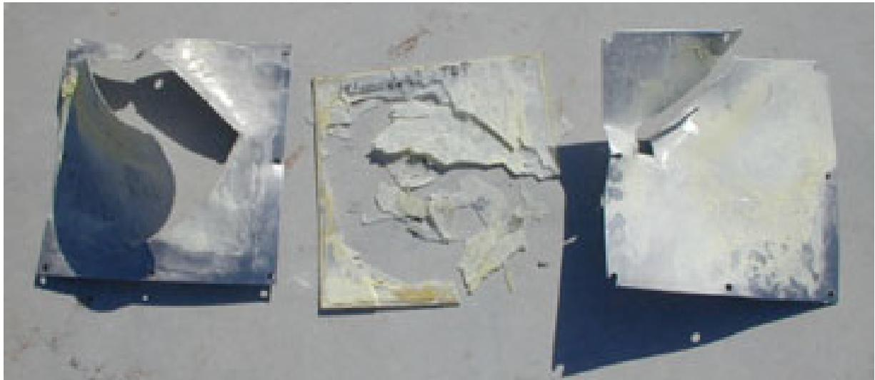
**Figure 9–13. Entire Contents of Enhanced Powder Panel Released During FAA Test in Which the Fire Was Prevented.**
