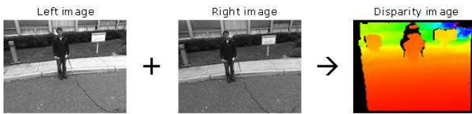
Fig. 2. Compute depth map from the stereo images.
