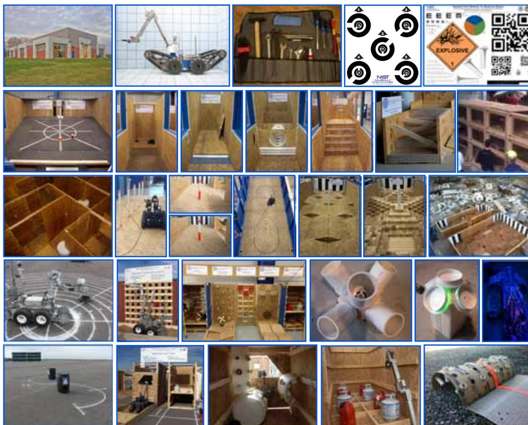
**FIGURE 2:** The suite of standard test apparatuses provide a breadth first approach toward testing. They rely on inexpensive materials that can be sourced around the world. They can be embedded into operational scenarios to provide measures of operator proficiency.
