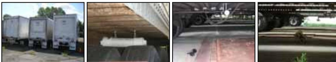
**FIGURE 26:** The *Trailer Underbody Reconnaissance* task included nine tractor trailers parked side-by-side. Ten visual acuity targets and ten objects of interest were placed on the underside of the trailers, one under each trailer with two under one particular trailer. Three operator stand-off positions were available depending on radio communications capability of the robot: 10m line-of-site, 75m line-of-sight, and 100m non-line-of-sight.
