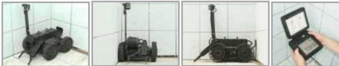
Figure 40) Armadillo-Manipulator-Wheels, MacroUSA Corp. and RE<sup>2</sup>, Inc., USA (4.8kg / 10.6lbs)
