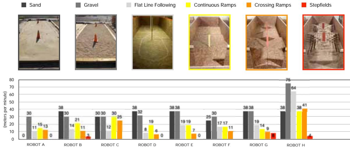
**FIGURE 46:** An example of bar charts generated from the performance data shows the comparison across a class of robots on increasingly complex terrains. Missing bars mean the robot abstained from the test method. Sponsors get charts with all the robot names identified. Robot developers get the same charts with only their robot name identified, providing a clear indication of their capabilities within the class.
