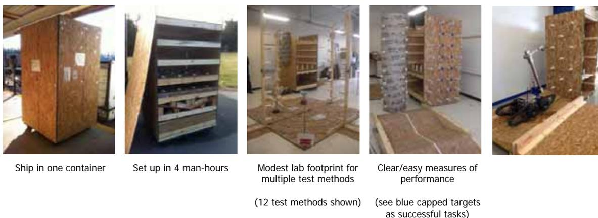
**FIGURE 18:** A sample set of training test methods in a box can contain introductory tasks or rather advanced tasks targetted for specific responder communities. For example, package capable bomb squad robots or C-VBIED tasks.
