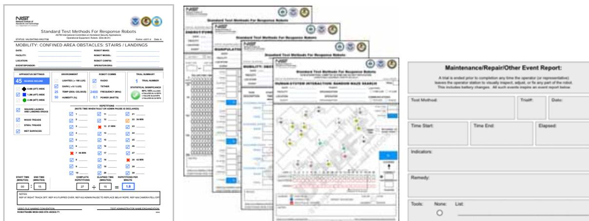
**FIGURE 14: A) A sample test form showing successful repetitions in blue check marks and anomalies in red Xs within a 30 repetition trial. B) Examples of other data collection forms designed to convey capabilities and anomalies graphically. C) Each Field Maintenance Reset inspires a separate form to capture the indications of the issue, the remedy implemented, the tools used if any, and the total time needed for the repair.**
