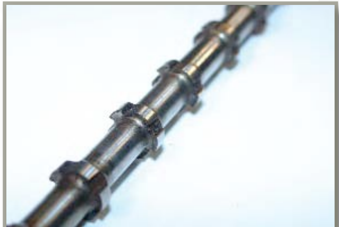
A gang broach that progressively cuts rifling in a barrel.
