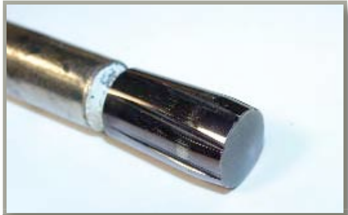
A button swage used to form rifling in a barrel.
