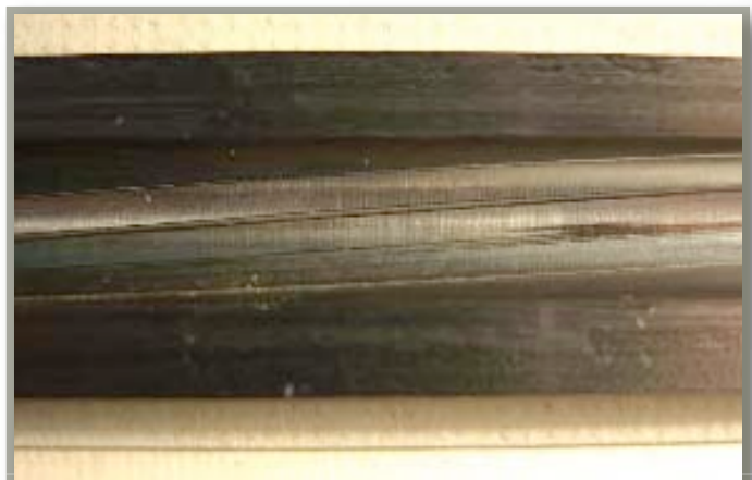
Cross section of a barrel showing toolmarks that survive the rifling procedure.
