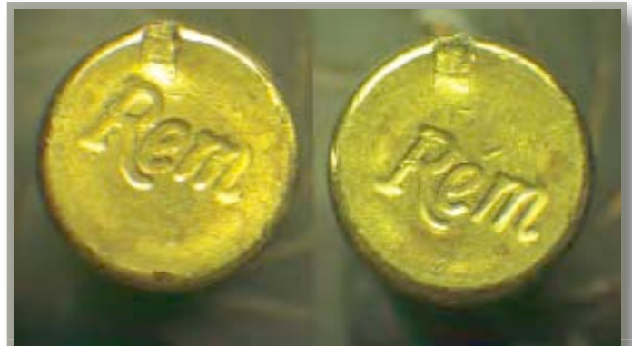
Firing pin impression comparison of two fired .22 caliber cartridge cases.
