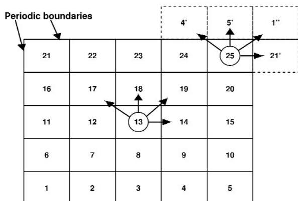
Fig. 2. Schematic 2-D representation of the link-cell algorithm.
