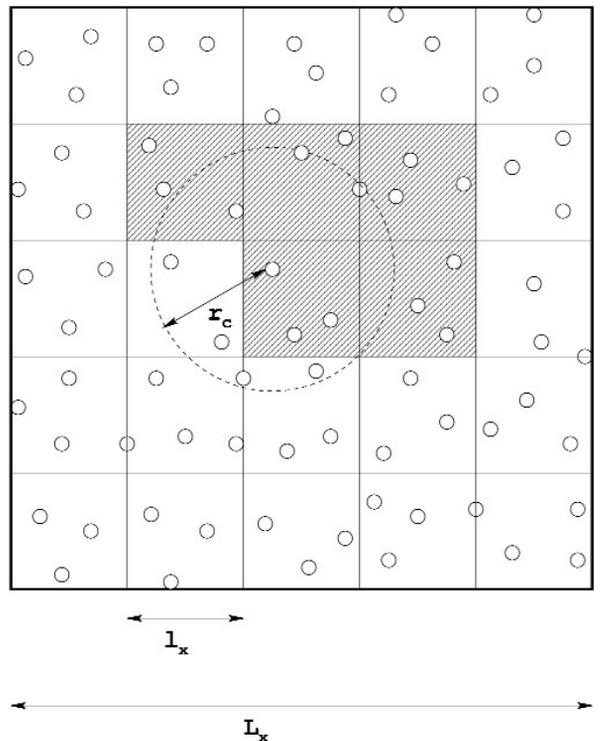
Fig. 1. Schematic diagram of link-cell algorithm for a two dimensional system (after Tildesley, Pinches, and Smith [11]).
