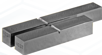
Figure 1. Examples of Charpy and Izod samples.
