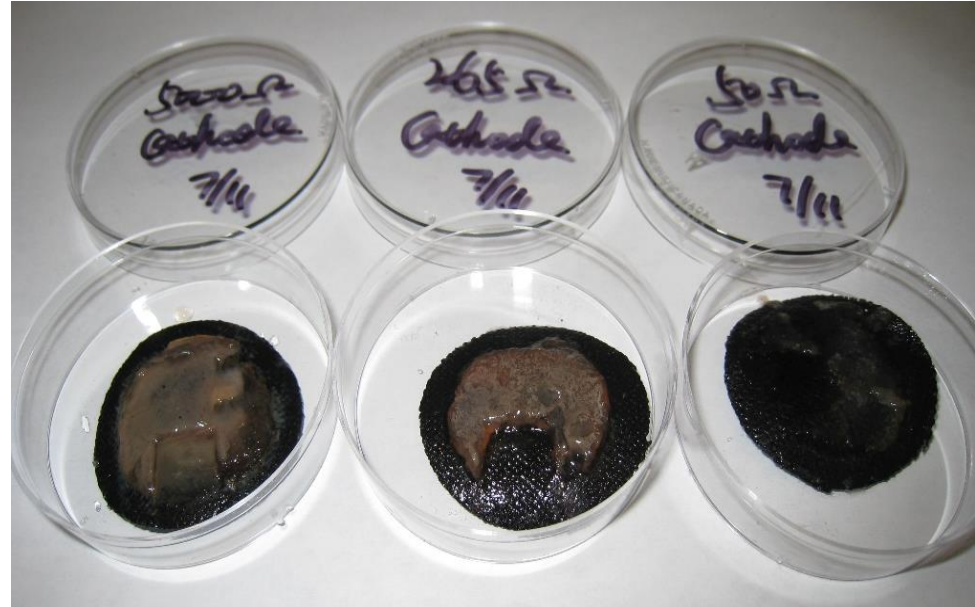
Cathode Biofilm After 6-month operation under different external resistors
