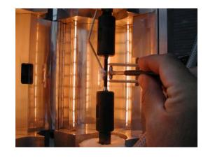
The servo-hydraulic machines are capable of fatigue testing at rates up to 20 or 30 Hz at 1 MN. These frames are equipped with state-of-the-art digital controllers for machine control and data analysis.
