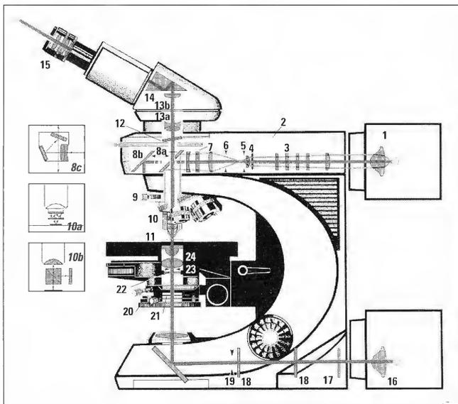
Cross-section diagram of DAS Mikroskop Leica DMLM
