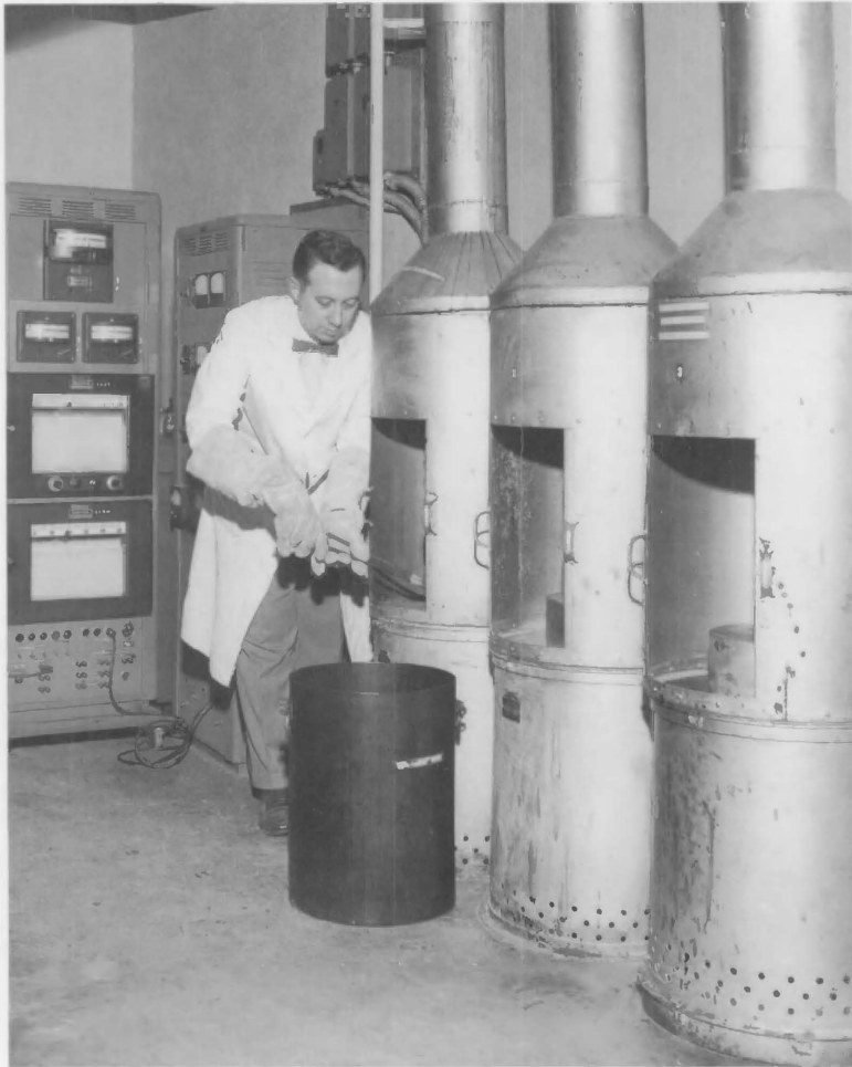
Melvin R. Meyerson of the NBS Metallurgy Division removed type 52100 tool-steel gage blocks from a chloride bath where they were immersed at 1550 °F for 15 min.
