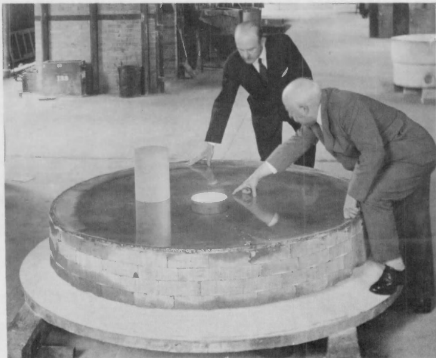
Prof. Clifford C. Crump, director of the Perkins Observatory and Dr. Burgess examining the Bureau's 69.5-inch telescope disk after an 8-inch hole had been drilled through its center for mounting. The disk after polishing was set up in the observatory at Ohio Wesleyan University.
