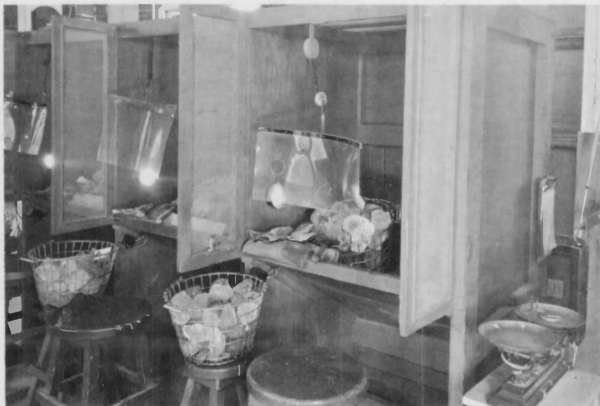
Quartz crystal inspection and testing laboratory, through which more than 6 million pounds of the crystals passed. These are 1-pound raw pieces, from which the small oscillator plates needed in radio and other electronic equipment will be cut.
