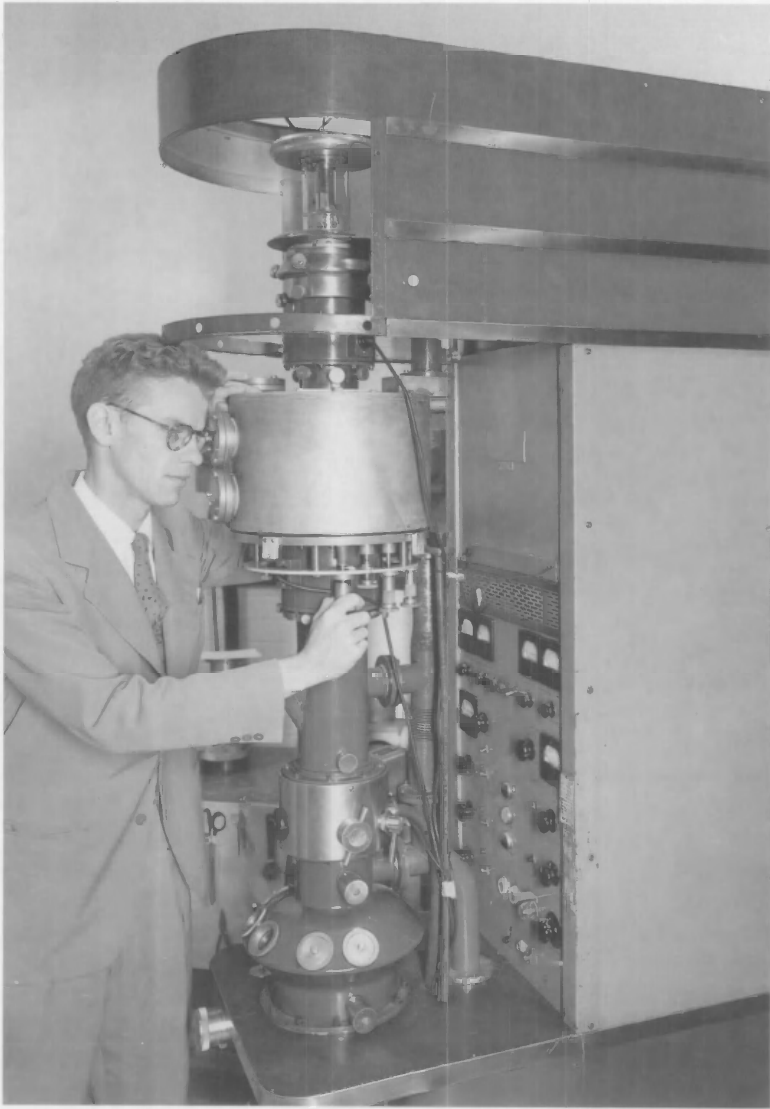
John Simpson adjusted an electron-beam interferometer, a device that utilized electron beams to produce interference fringes in much the same way that conventional optical interferometers used light beams. The instrument employed diffraction from an extremely thin crystal as a means for splitting and recombining an electron beam. Three crystals were mounted in a vacuum chamber (center) placed between the illuminating and viewing systems of a conventional electron microscope. Each of the crystal mounts could be rotated around the optical axis. The mount of the first crystal could also be translated along the optical axis. The controls for these motions were brought out from the bottom of the evacuated chamber.
