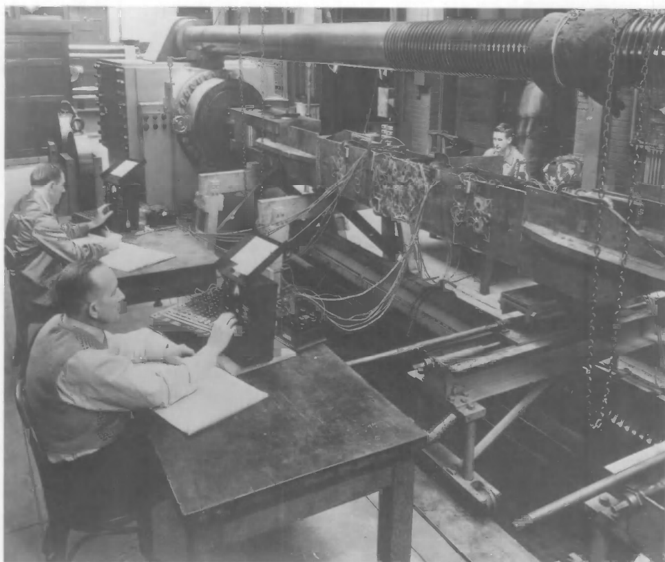
NBS staff from the Metallurgy Division took data during a tensile test at room temperature of an interrupted longitudinal specimen from a ship plate.
