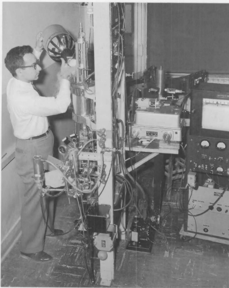
View of the equipment used at NBS in the low-temperature stabilization of free radicals. Arnold M. Bass added liquid nitrogen to the outer Dewar of the cryostat in which the free radicals were frozen into solid form. The spectroscopic equipment at right was used to study and analyze the visible and ultraviolet radiation given off by the frozen atoms.
