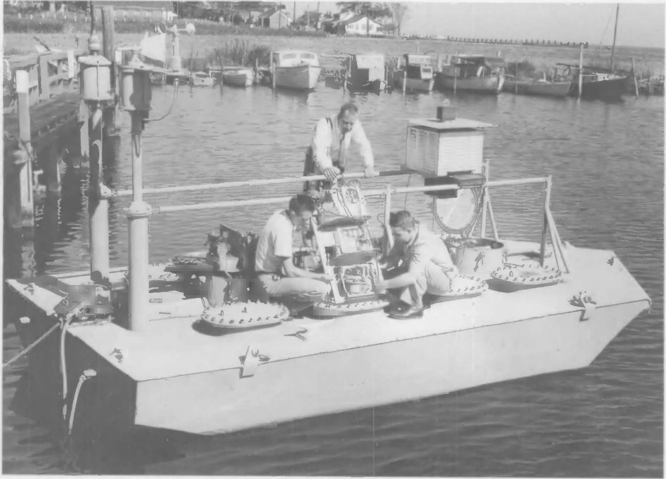
This ocean-based weather station developed by NBS automatically reported local weather data by radio. It could be anchored in a remote location and left unattended for as long as six months.
