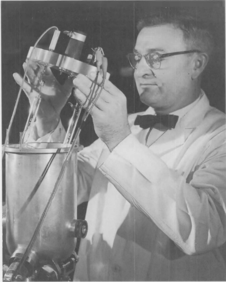
Karl F. Nefflen of the Engineering Metrology Section assembled a krypton-86 lamp. The lamp was maintained at the triple point temperature of nitrogen, 63 K, to improve the reproducibility of the standard wavelength.
