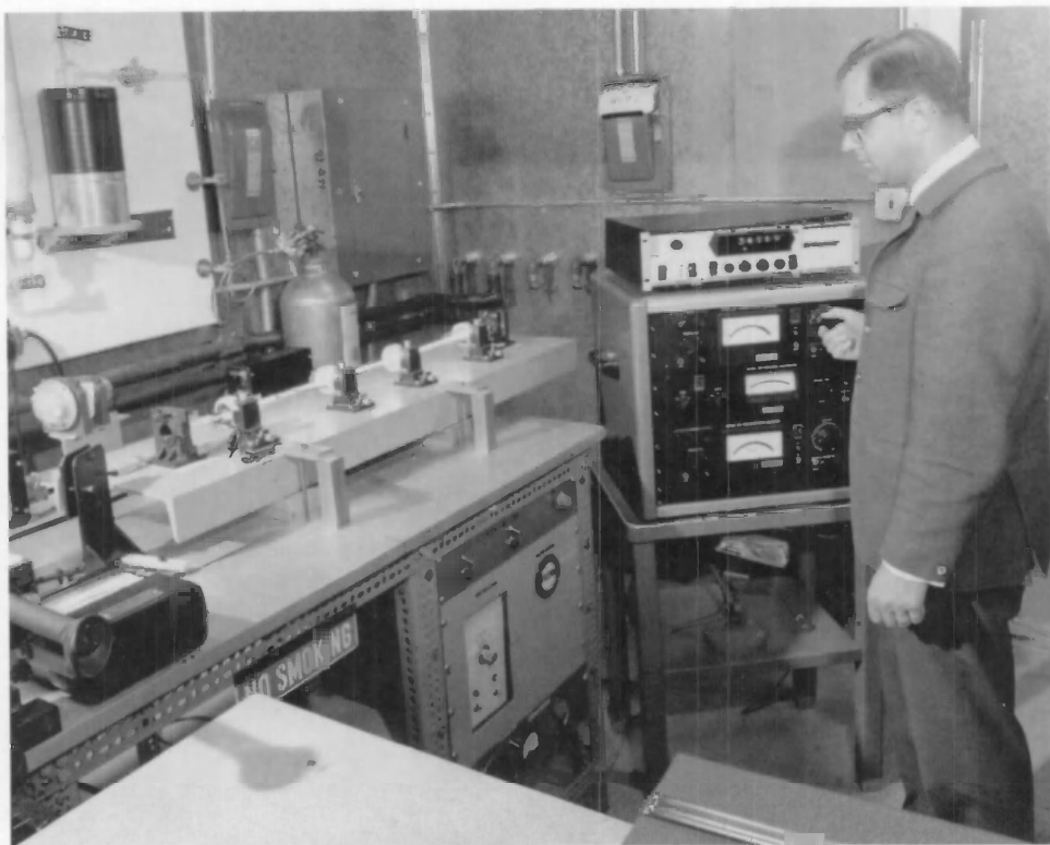
Gerhart J. Kneissl obtained reflectance measurements from the laser-source reflectometer. The laser beam was alternately directed into a large integrating sphere (outside picture at left) and a small averaging sphere (left center). Reflectance values were indicated by a digital voltmeter.
