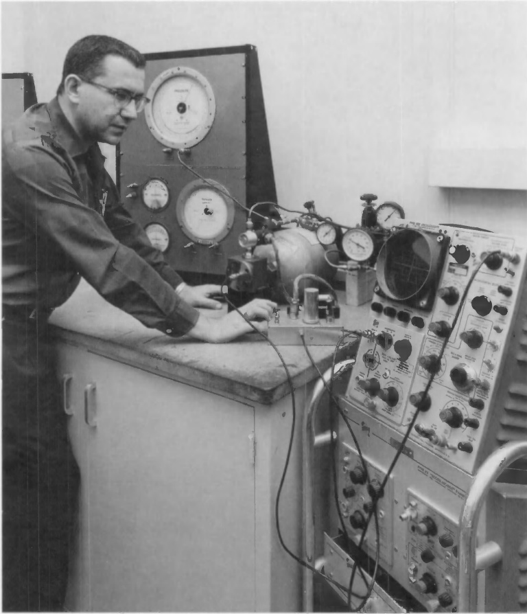
The Bureau developed a number of techniques and devices for calibrating and evaluating transducers within the Interagency Transducer Project. In this photograph, NBS engineer Paul Lederer prepared to trigger a pneumatic step-function calibrator.
