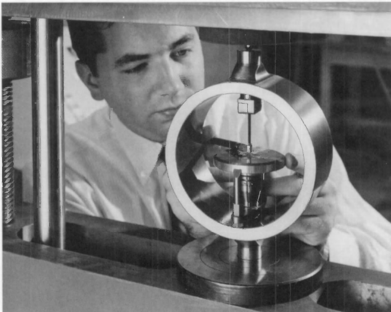
Arnold J. Mallinger inspected a proving ring before its calibration as a force standard in a deadweight machine at the National Bureau of Standards.
