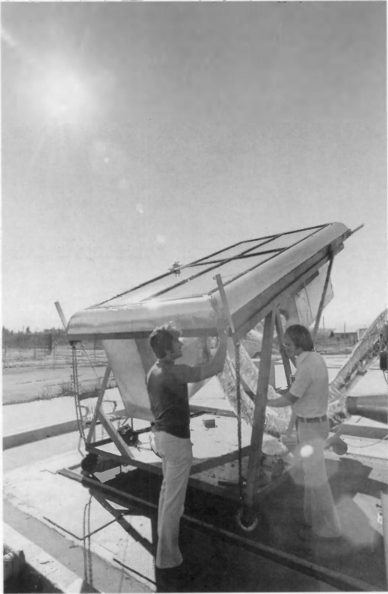
At a former NIKE missile base adjacent to its Gaithersburg site, NBS engineers tested solar collectors in a project sponsored by the Energy Research and Development Administration. A key part of solar heating and cooling systems, the collectors were lowered into the former missile silos when not under test.
