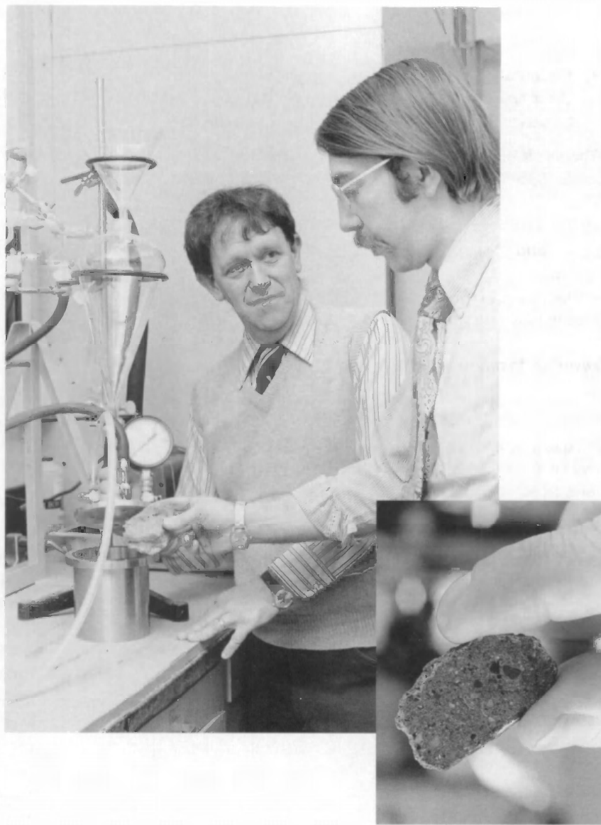
Chemist James R. Clifton of the Bureau's Center for Building Technology headed an NBS project on preservation technology which was initiated at the request of the National Park Service. In the accompanying photograph, Clifton (left) and Paul Brown prepared an adobe specimen for microscopic examination by impregnating it with methyl methacrylate. The inset shows a cross section of an adobe specimen.
