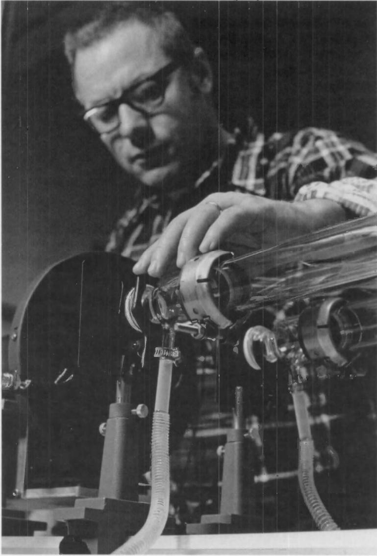
NBS researcher Albert E. Ledford adjusted an instrument developed at the Bureau to measure very small amounts of ozone, a serious pollutant at ground level but protector against ultraviolet radiation in the upper atmosphere.
