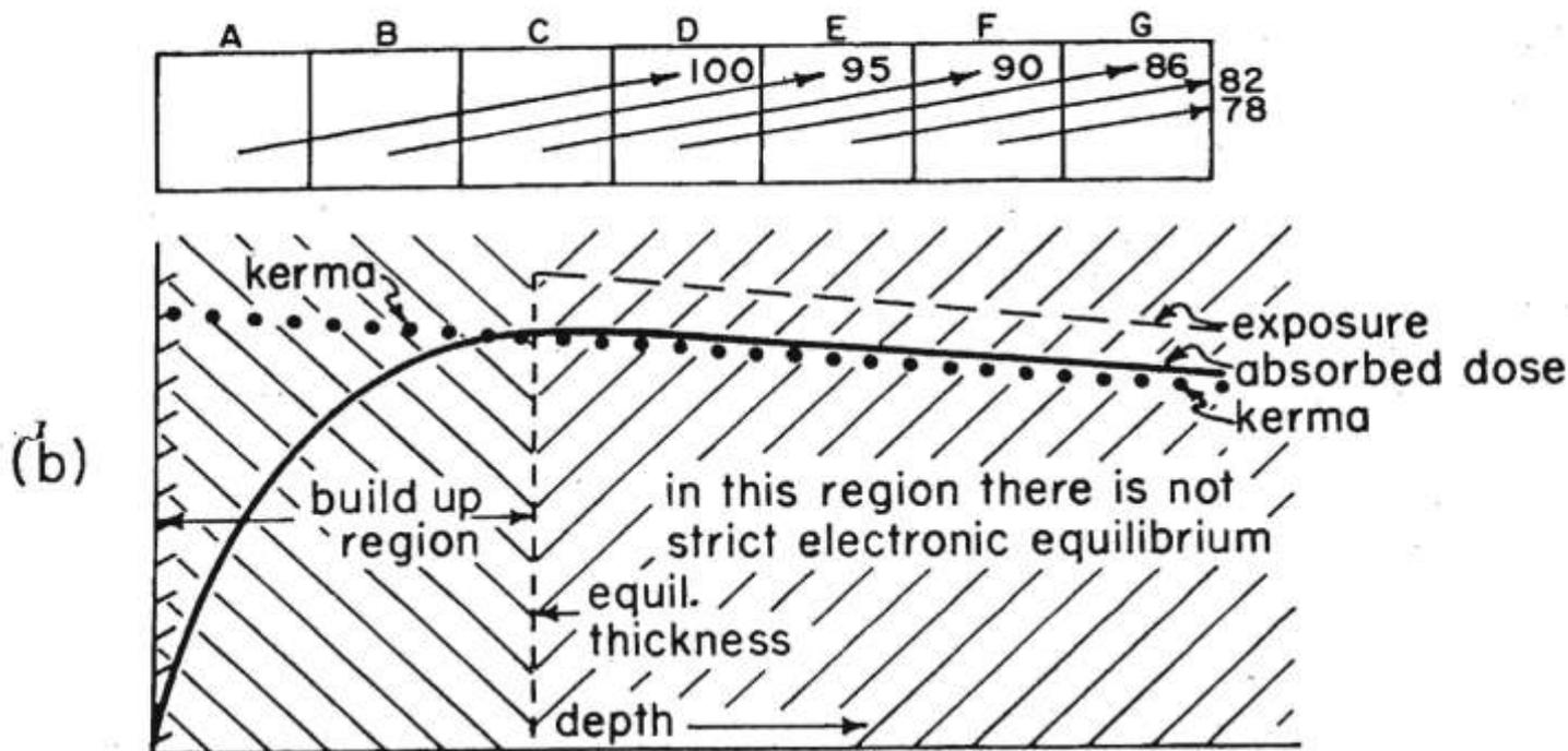
FIGURE IX-3.(a) Graph showing schematically why the absorbed dose increases with depth and how electronic equilibrium is achieved when there is no attenuation of the primary. (b) Graph as (a) when attenuation of the primary occurs. Now electronic equilibrium is not produced even at depths beyond the equilibrium thickness. Kerma and absorbed dose have the same units and so the curves are comparable; exposure is in different units and is not comparable.
