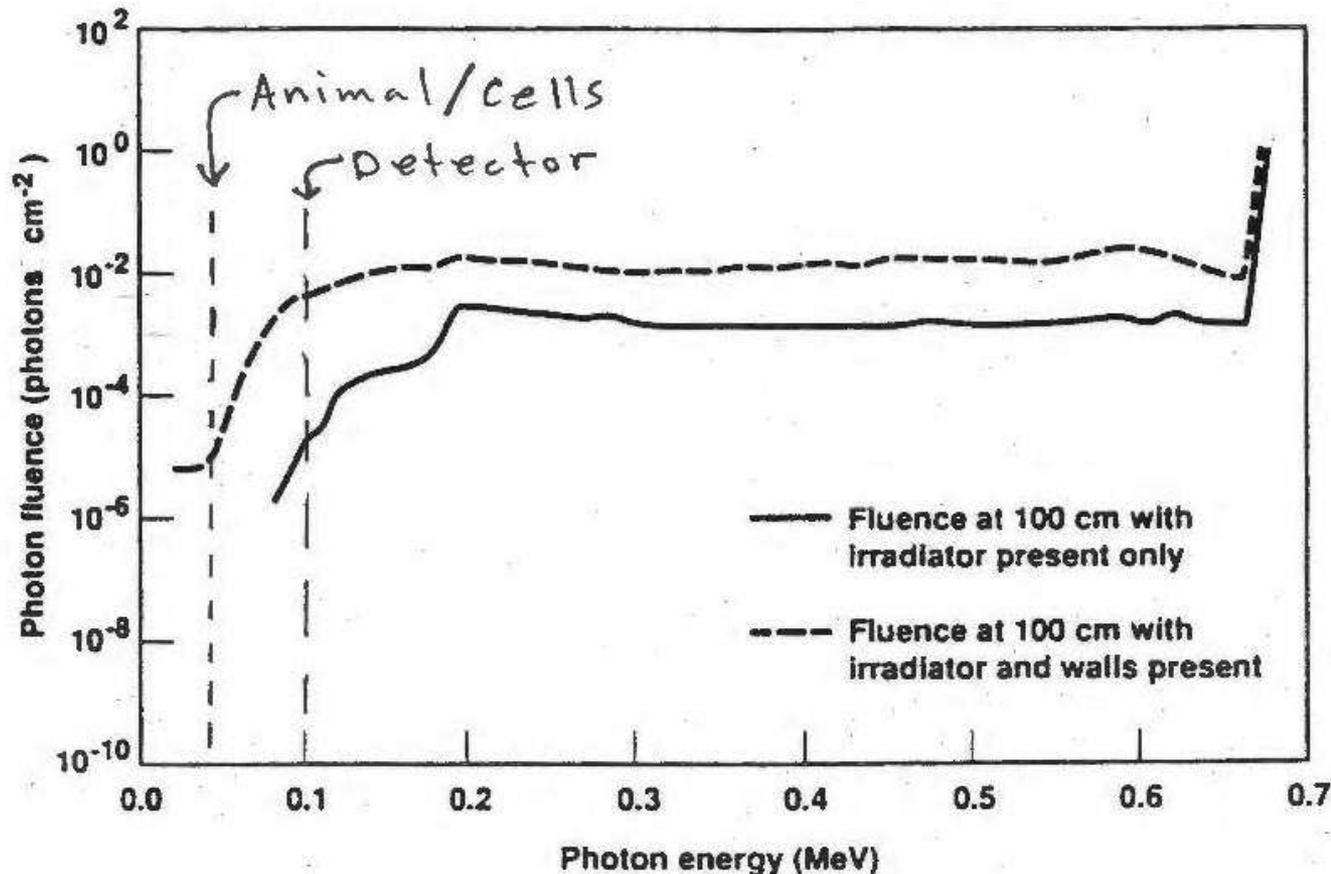
Fig. 5. Calculated photon energy spectra showing additional low-energy scatter contributed by the irradiator and the room walls.
