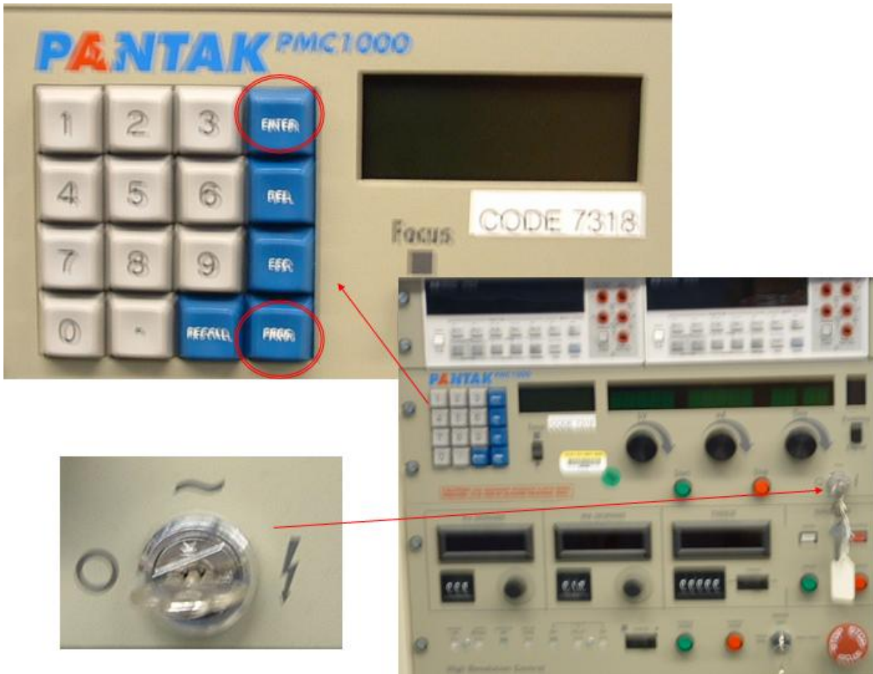
Figure 6. 100-300 kV x-ray controls.
