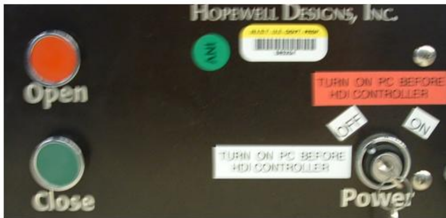
Figure 7. 100-300kV control panel and range control.
