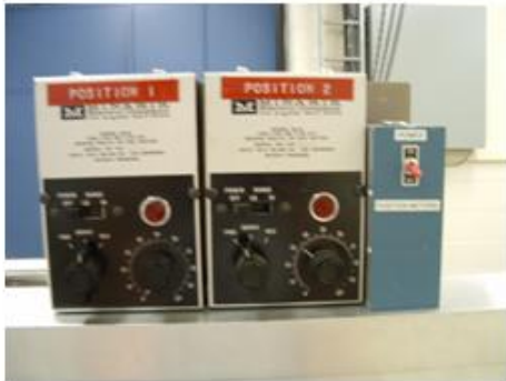
Chamber alignment controls 300 kV range
