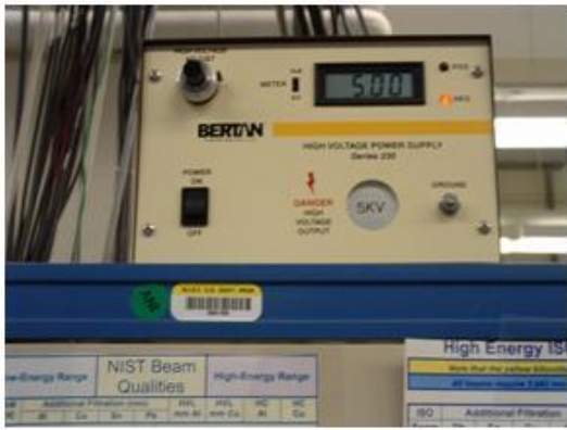
Figure 8. 100-300 kV high voltage power supplies.
