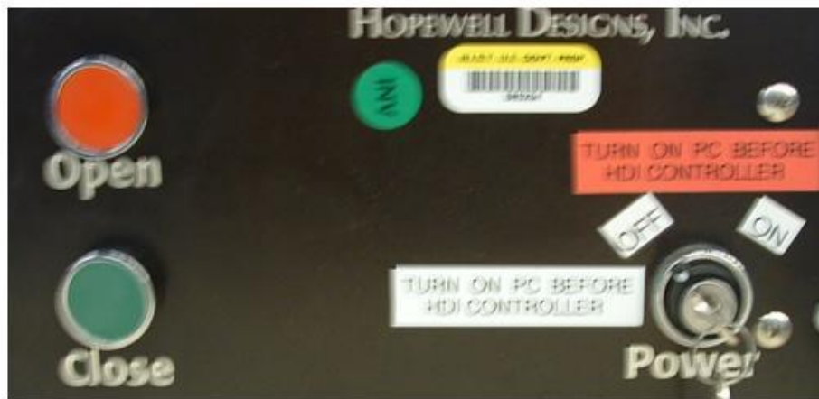
Figure 7. 100-300kV control panel and range control.
