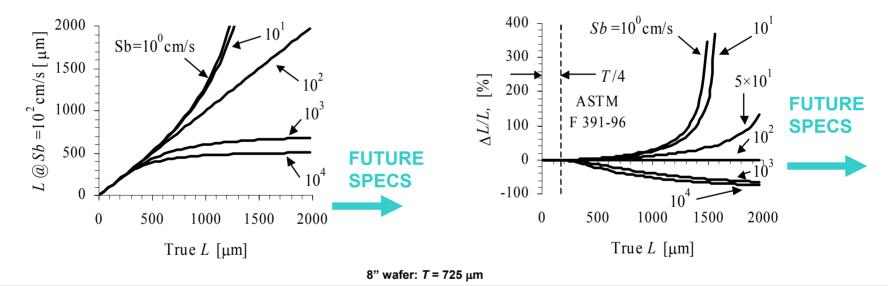
Back-surface recombination affects the accuracy of diffusion length measurements and becomes more significant at higher values of diffusion lengths
