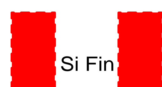
Figure 1. (a) Representation of SOI (silicon on insulator) fin structure cross section with sidewall roughness. The arguments for this paper apply just as well to bulk fins.
