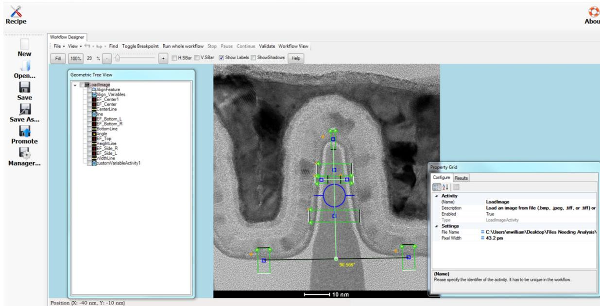
The recipe designer also contains a geometric view with separate windows related to A, B, and C above (A and B not shown). The geometric view allows one to visually place metrology activities on to a relevant image (A). This view also provides the ability to run metrology recipes offline with a rerun images function. In addition to offline metrology this functionality is useful for optimizing metrology recipes.
