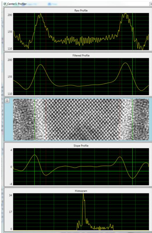
Many parameters are available for optimizing metrology recipes. The image on the left shows a profiler associated with a double edge finder. Algorithms are available to determine edge placement based on intensity values or the slopes of those intensity values. It is also possible to adjust the smoothing of the raw profiles and to add weighting to the probable region within the edgfinder where the edge will be found.
