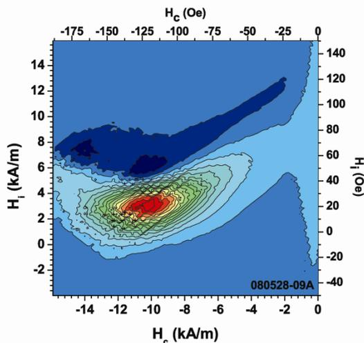
Figure 2.2: FORC diagram that shows the density of magnetic domain switching as a function of the coercive and interaction fields.
