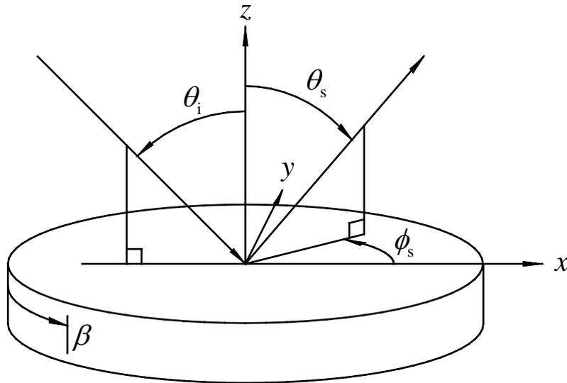
**FIGURE 1** The scattering geometry and angle convention used by the calculations. The incident angle is  $\theta_i$ . The scattering direction is defined by polar angle  $\theta_s$  and azimuth angle  $\phi_s$ .
