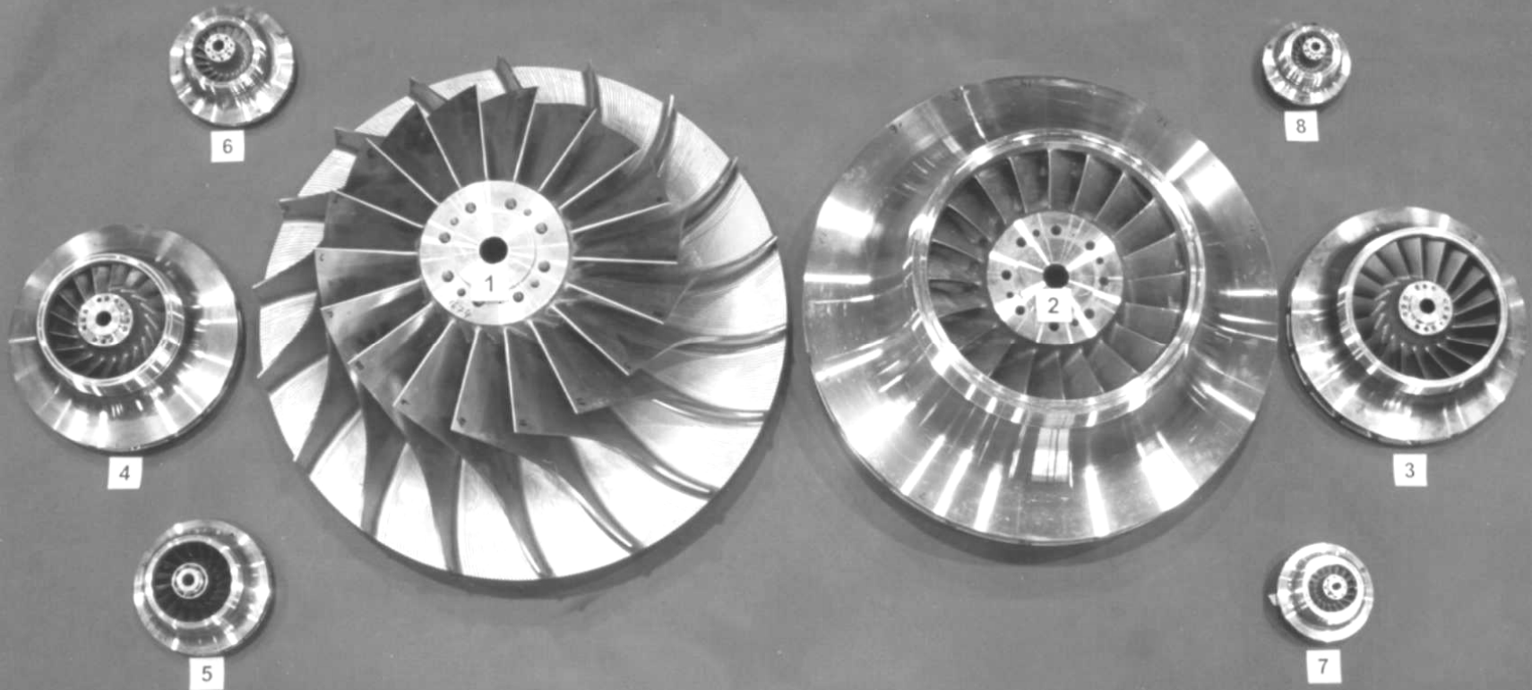
Integrally Geared Centrifugal Impellers: Stages 1 through 8
