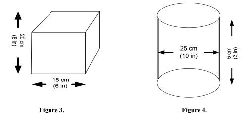
(b) in the case of a cylindrical or nearly cylindrical container, 40 % of the product of the height of the container times the circumference;
