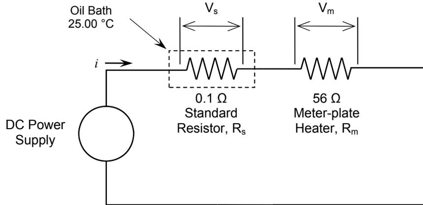
Figure A1. Electrical schematic for meter-plate power measurement.
