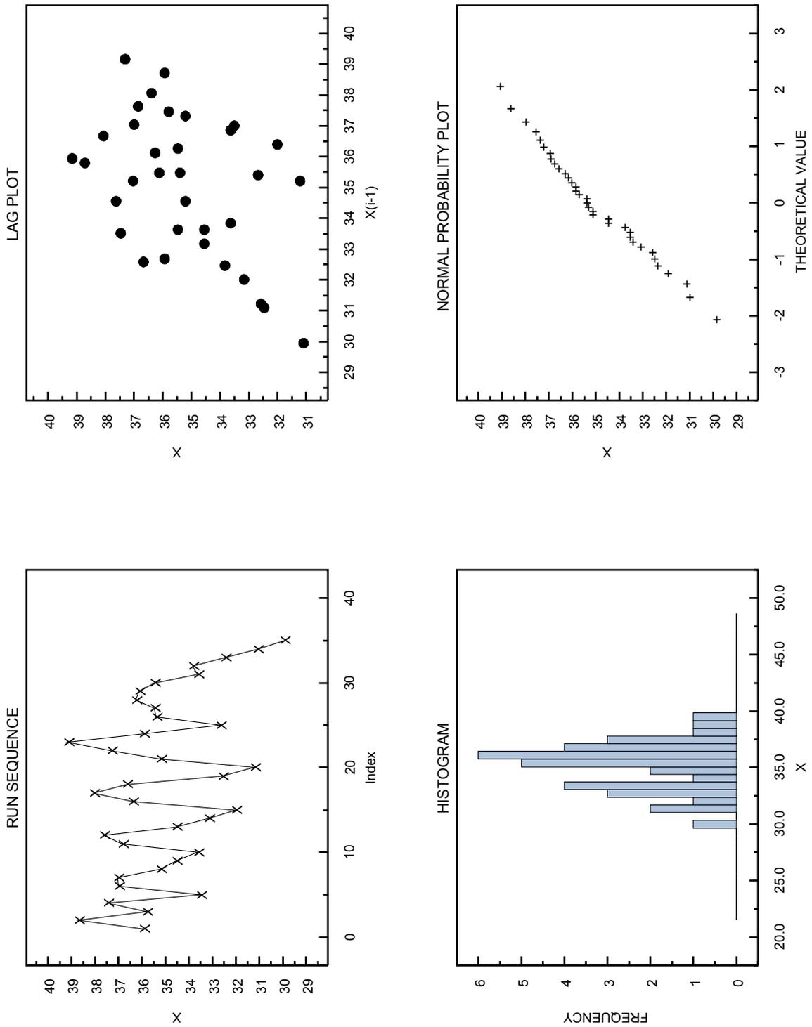
Figure 5. Graphical analysis of bulk density measurements ( $n = 35$ ) from Board 049: (a) run sequence plot, (b) lag plot, (c) histogram, (d) normal probability plot (normality index). Summary statistics: sample mean =  $35.09 \text{ kg/m}^3$ , sample standard deviation =  $2.26 \text{ kg/m}^3$ .
