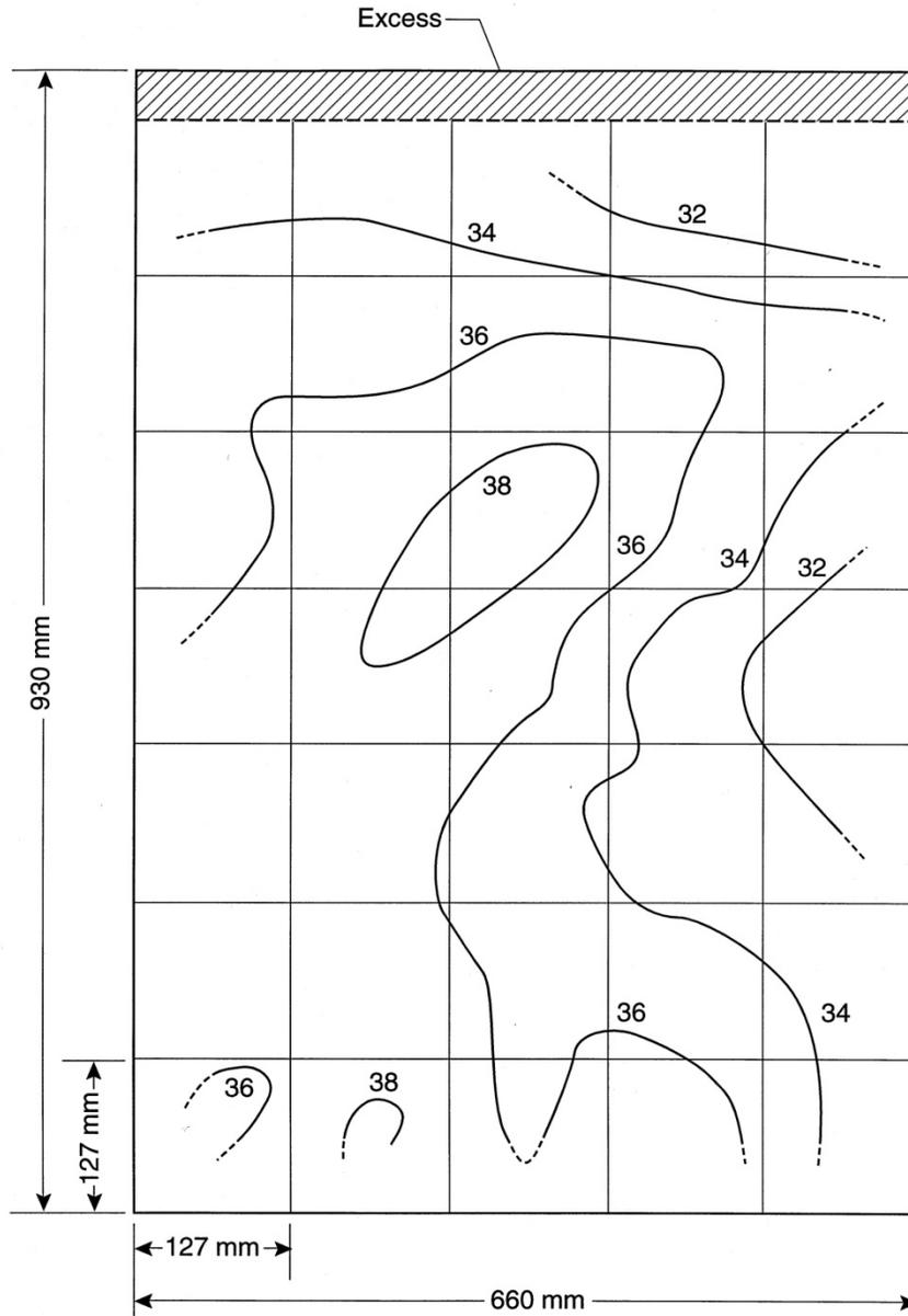
Figure 6. Contour plot of bulk density (in  $\text{kg/m}^3$ ) for Board 049.
