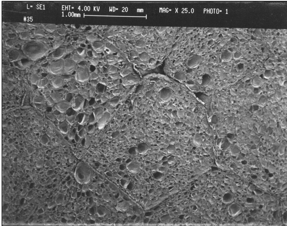
Figure 7a. SEM micrograph (25×) shows outlines of molded beads and internal cellular structure
