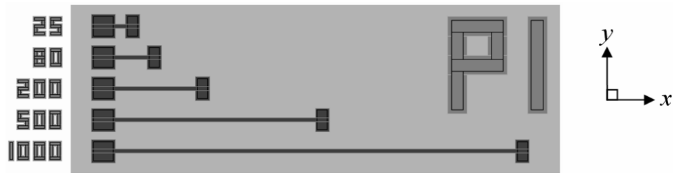
Figure L6. Poly1 fixed-fixed beam test structures for in-plane length measurements on the round robin test chip.
