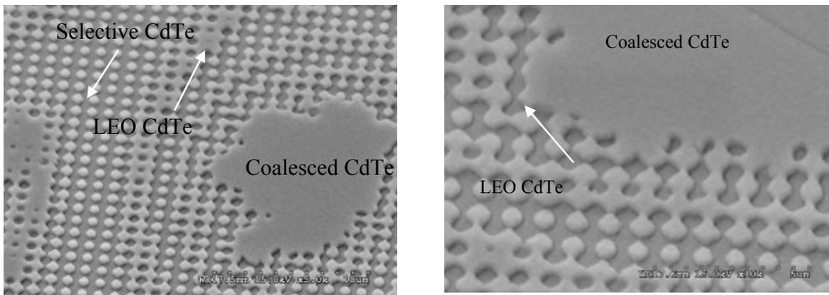
Figure 3: LEO and coalescence of CdTe on nanopatterned SOI substrates.
