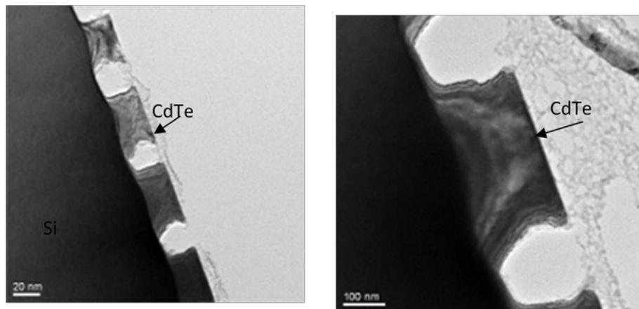
Figure 5: Two low resolution cross-sectional TEM images of CdTe grown on nanopatterned CdTe buffer layers
