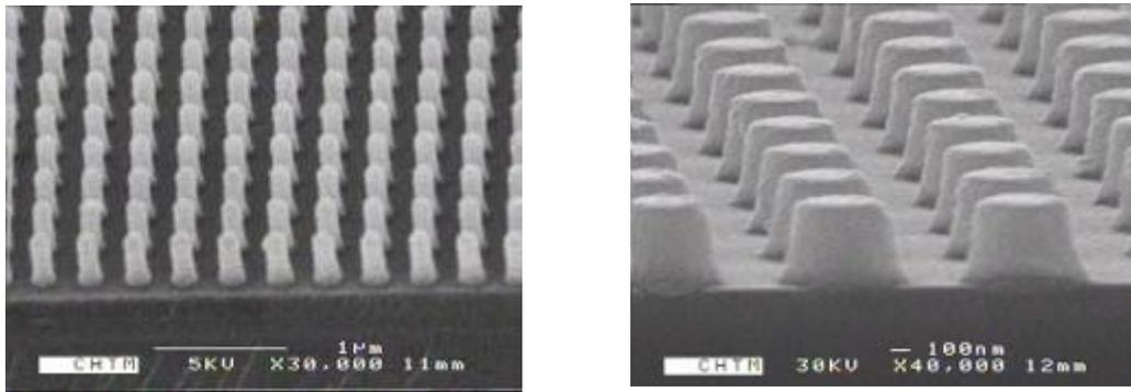
Figure 1: Cross-sectional SEM image of 500 nm pitch grating (left) and 360 nm pitch grating (right)
