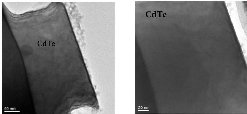
Figure 6: Two high magnification TEM images of CdTe regrown on nanopatterned CdTe buffer layers.
