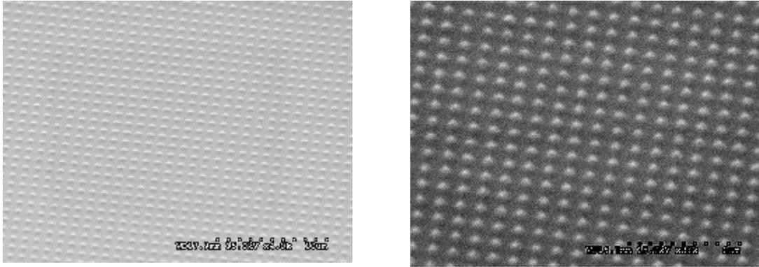
Figure 2: Two plan view SEM images of CdTe selectively grown on nanopatterned SOI substrate
