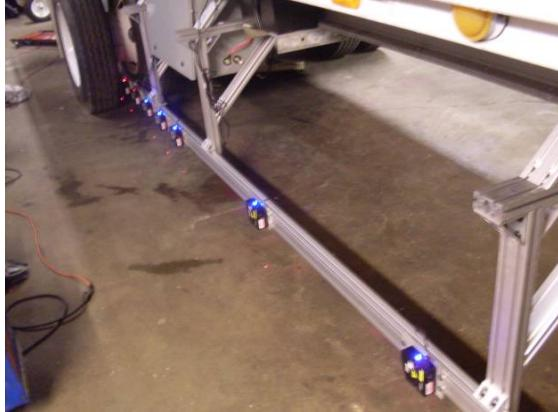
Fig. 4<sub>a</sub>. Eight lasers are mounted on the beam
