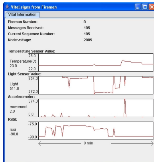
Figure 5.2: Vital signs GUI to display the sensor readings of the first responder.
