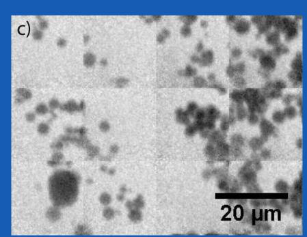
**Fig. 2:** (a) simulated and (b) measured images in the image plane. The simulation does only consider zero and first order diffraction of the MLL, but the general shape of the illumination is well predicted. (c) A stitched radiograph of a particle array demonstrates the suitability of the condenser optics for full-field XRM.
