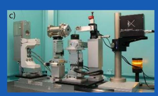
**Fig. 1:** (a) An MLL can be understood as linear zone plate consisting of several thousand individual layers. Two MLLs are assembled to achieve a 2D focusing or imaging behavior. (b) Optical path of a full-field XRM with a multilayer mirror and crossed MLLs. The image generated by first order diffraction separates in the image plane from other orders. (c) Experimental setup with a conventional X-ray microfocus source and X-ray detector.
