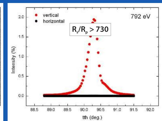
Fig. 4: Characterization of the fabricated mirrors at 792 eV. To obtain the Brewster angle of  $2\theta \approx 90^{\circ}$  at this photon energy, a multilayer period of d = 1.1 nm is required. An excellent  $R_s/R_p$  ratio of > 730 was achieved.
